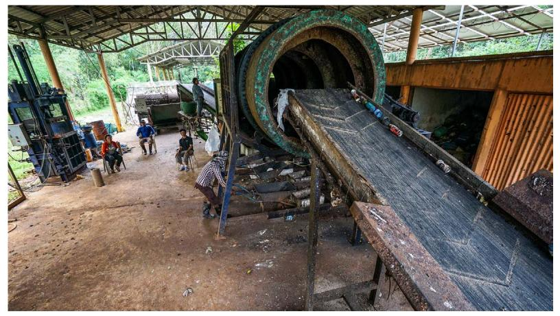
the waste sorting machine and deposited into containers below. Portions of it will be placed in a fermentation tank for biogas production that can be used for home cooking. Other parts will be turned into fertiliser that can be used for organic gardening on the island.
